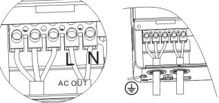
**Note:** The grounding wire shall be as thick as possible (cross-sectional area is not less than 4mm2). The grounding point shall be as close as possible to the all-in-one solar charge inverter. The shorter the grounding wire, the better.
